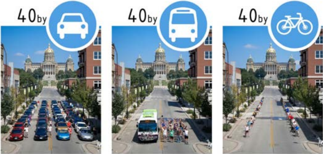
Amount of space required to transport the same number of passengers by car, bus, or bicycle.
